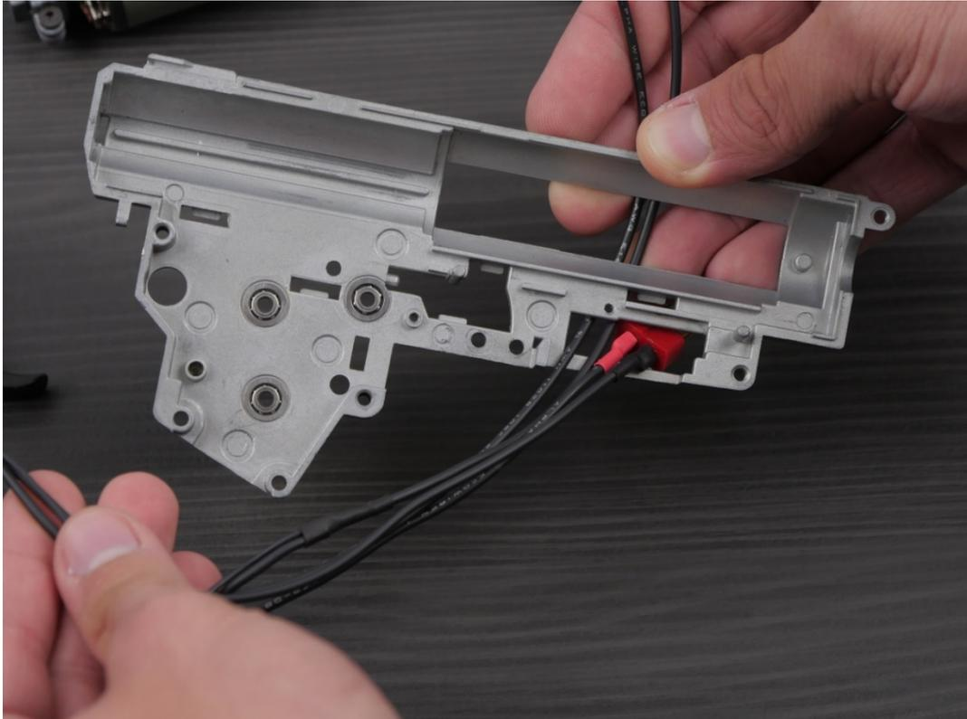
2.2 Place the wires in gearbox shell so as the unit can fit properly without any resistance.
