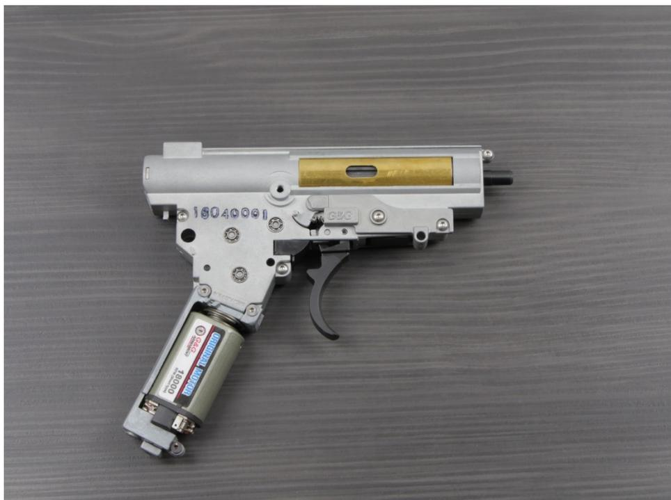
1.1 Disassemble the motor.
