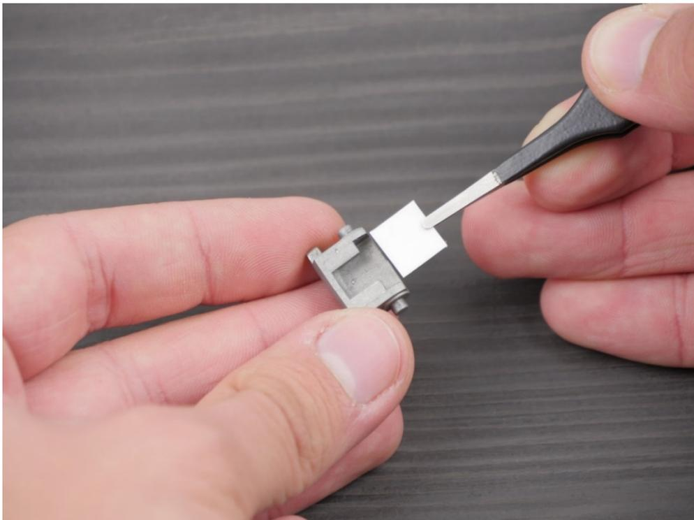
4.4 After pasting the first sticker, assemble both trigger elements and estimate the clearance between them. If you feel that there is any, you can use next stickers. Remember that trigger should work smoothly.
