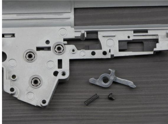
1.5 Clean the gearbox case using solvent.
