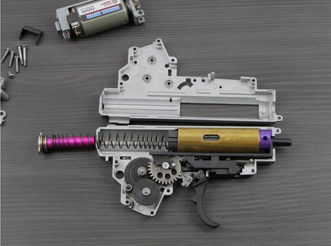
1.4 Disassemble all the internal parts (cylinder set, spring with spring guide, gears with anti-reversal latch, trigger, trigger switch, cut-off lever with spring).
