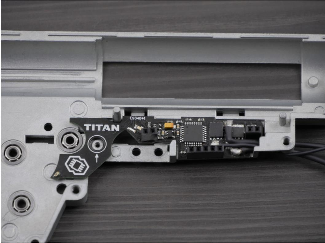
2.4 If the bottom board fits correctly, use the cut-off lever screw to stabilize the unit. Use also the included washers.
