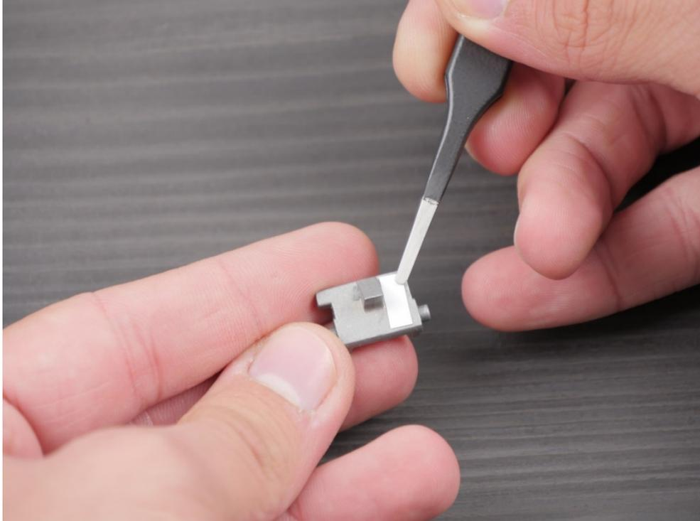
4.3 Paste one Trigger anti-backlash sticker inside the moving element of the trigger.
