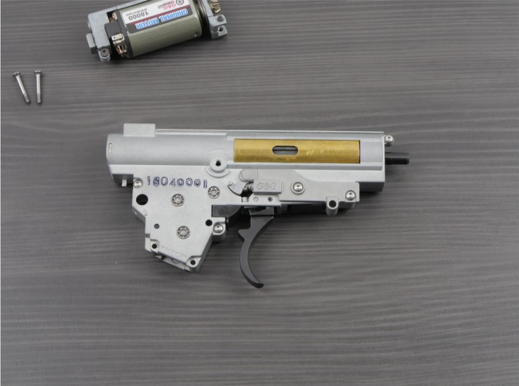
6. After installing the remaining gearbox external components, go to the wiring placement. You can use the picture below or your previous wiring as a suggestion.
