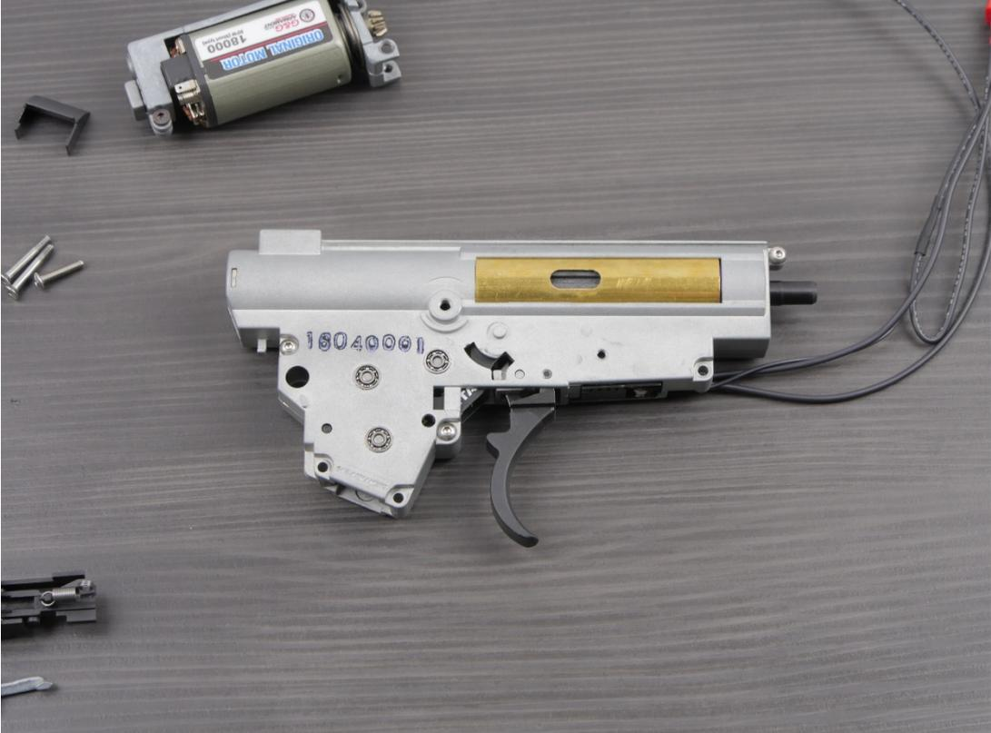
5.3 In some replicas (G36, UMP, etc.) you need to modify the mechanical trigger lock, because it is too long and touches the TITAN's top board. In this case, grind the protruding element by around 1.5/2mm.
