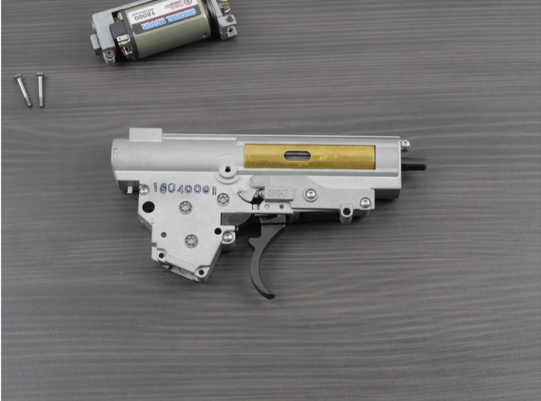
1.2. Dismantle the gearbox external parts (sector gear cover, trigger lock, screws).
