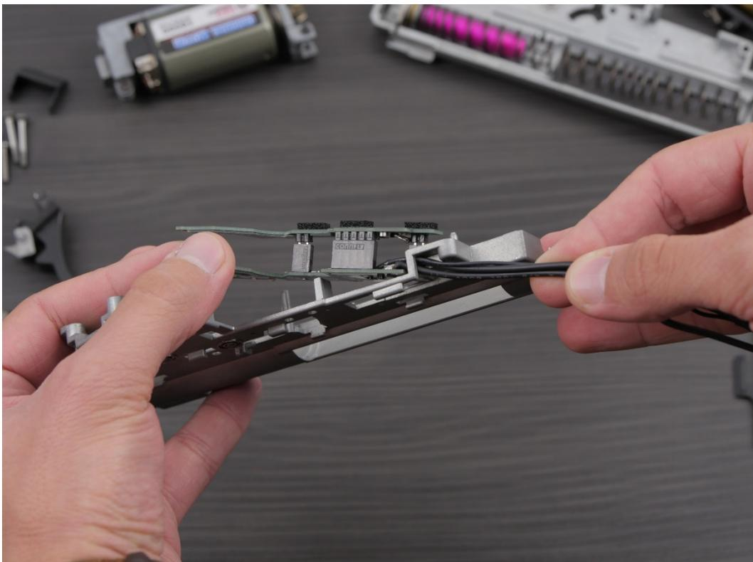
2.3 Carefully place the bottom board in the gearbox shell. TITAN V3 fits CNC gearboxes with very small backlash. While fitting TITAN, pull cables and at the same time push board in to right place.
